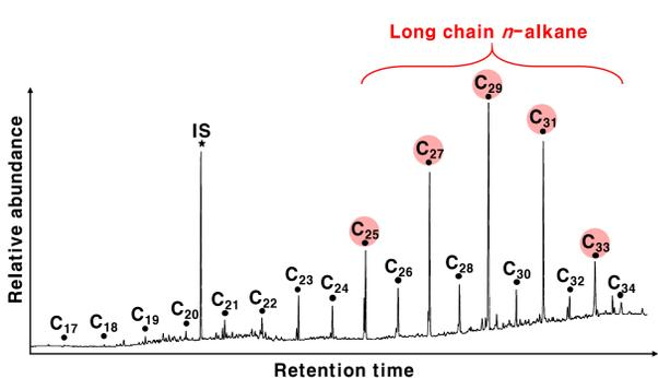
Fig. 2. An example of GC-FID chromatograms of *n*-alkanes ( $\text{C}_{17}$ - $\text{C}_{34}$ ) obtained from the sample EC1 2011/04/16\_2300m.
