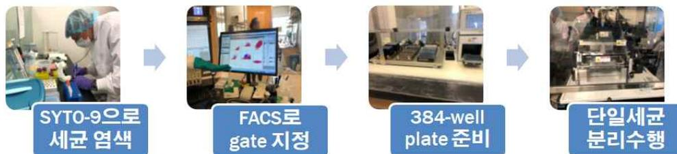
Figure 35. The experimental process conducted at the single cell genome center of the Bigelow Laboratory
