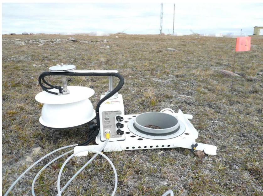
Fig. 8. Automated chamber (LI-8100-104, LI-COR).
