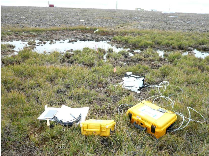
Fig. 7. Portable methane analyzer (UGGA, LGR) and a chamber system.
