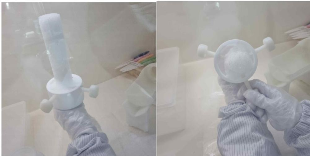
Fig 5.4. Inner layer with diameter of ~3 cm after chiselling for the depth sections between 6.2 to 9.8m
