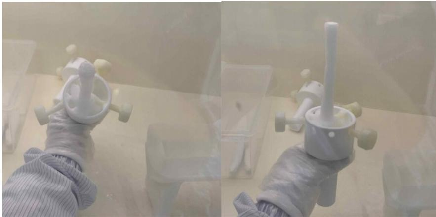
Fig 5.3. Inner layer with diameter of ~1-1.2 cm after chiselling for the depth sections between 4.2 to 6.2m
