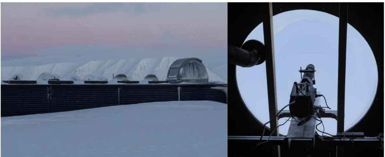
Fig. 16 All Sky Camera installed at KHO, Svalbard, Norway to observe aurora with 630.0nm, 557.7nm, 427.8nm filters near the polar cap/cusp region.
