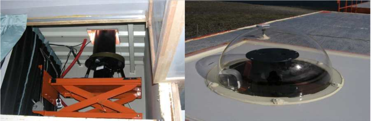
Fig. 5 Spectral Airglow Temperature Imager (SATI) at KSS. It measures airglow emissions occurring at the upper atmosphere to observe the temperature in the region.
