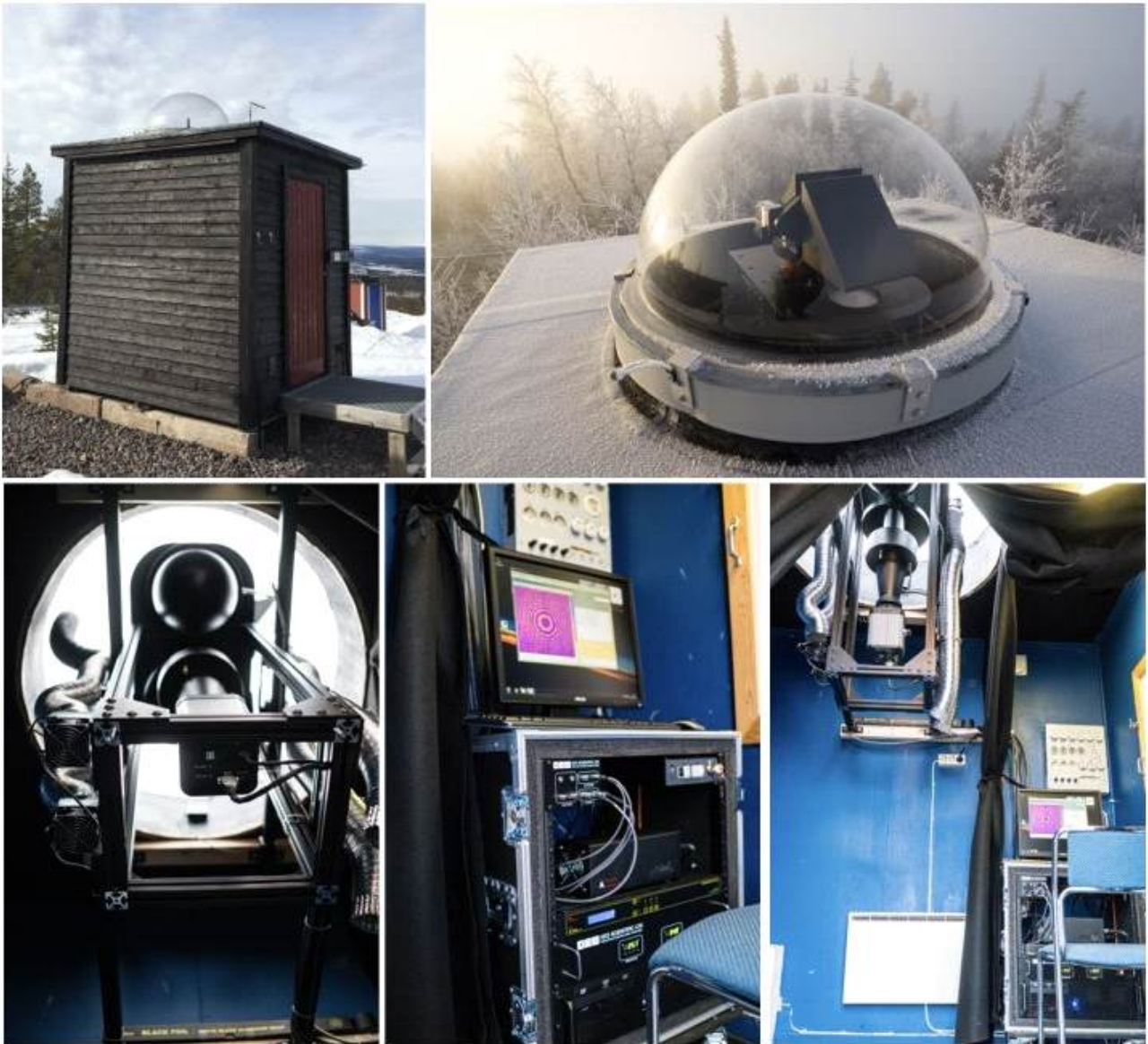
Fig. 15 Fabry-Perot Interferometer (FPI) installed at ESRANGE, Kiruna, Sweden in Oct. 2016 for the simultaneous observations for the neutral winds and ion drift in the auroral region.
