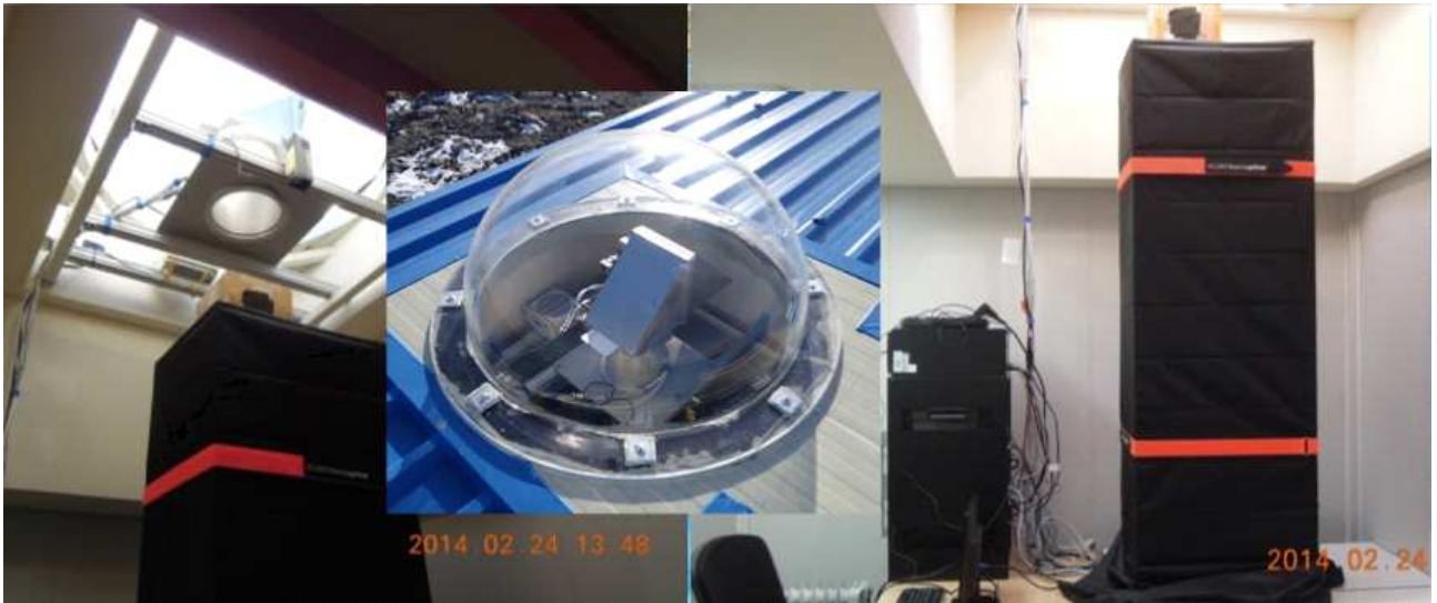
Fig. 9 Fabry-Perot Interferometer installed at Jang Bogo Station, Antarctica in March 2014 to observe the neutral winds and temperature in the polar upper atmosphere.
