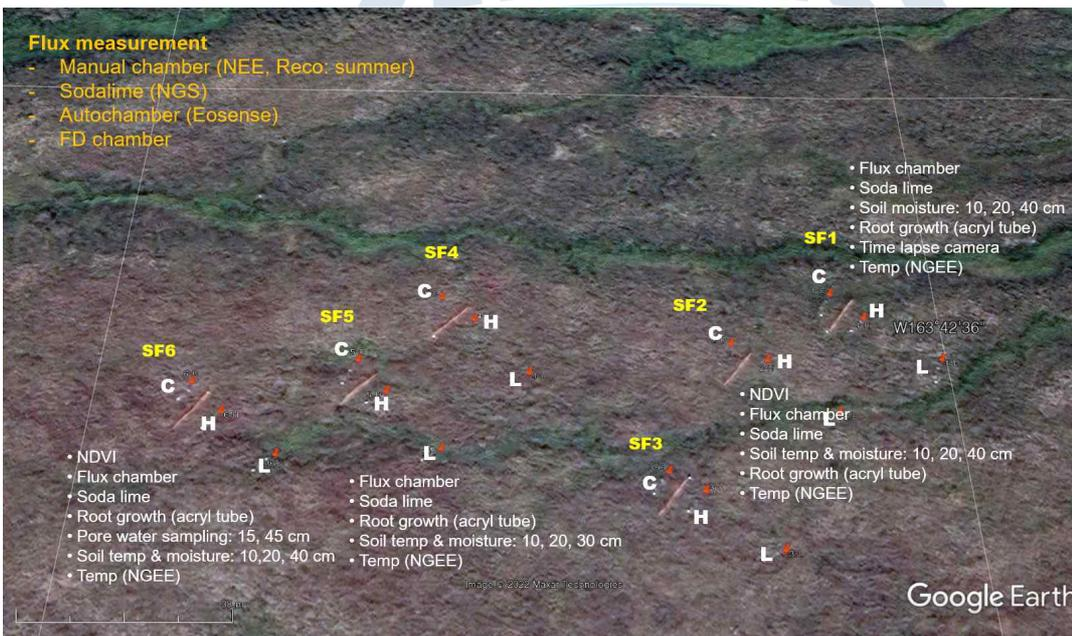
Fig. 2. Layout of snow fences and installed sensors for monitoring in Council, Alaska
