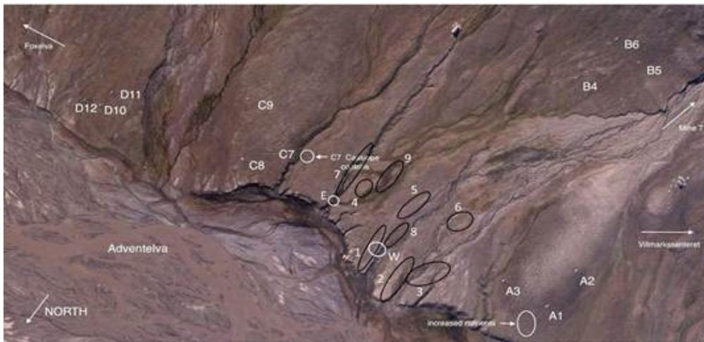
Fig. 15. Map displaying sites with experimental snow fences (A–D) and natural snow depth gradients (marked with ellipses 1–9).
