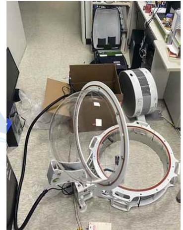
Fig. 4. The gas analyzer (Picarro G4301) and the connected auto chamber (eosAC-LT)
