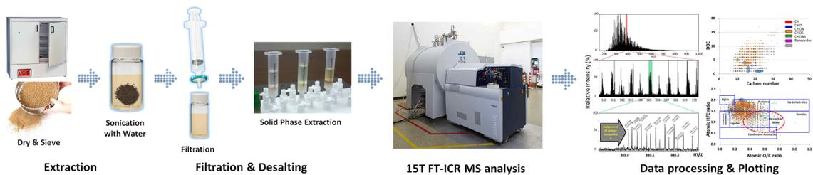
Fig. 26. Advanced analytical platform for characterizing chemical properties of soil organic matter using ultrahigh-resolution FT-ICR mass spectrometry.
