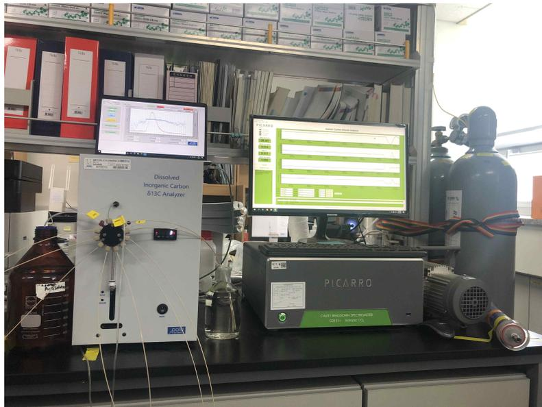
Fig. 3.3.1 Measurement system for dissolved inorganic carbon and d13C analysis.
