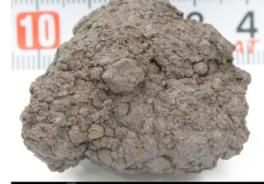
Figure 10. Photo and BSE image of the EET 15056(EL6) chondrite. The rock is heavily weathered. The weathering products such as iron oxides replace almost all Fe-Ni metal.
