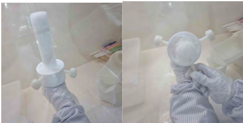
Fig 5.4. Inner layer with diameter of \sim 3 cm after chiselling for the depth sections between 6.2 to 9.8m
