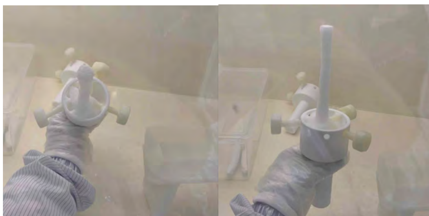
Fig 5.3. Inner layer with diameter of \sim 1\text{--}1.2 cm after chiselling for the depth sections between 4.2 to 6.2m
