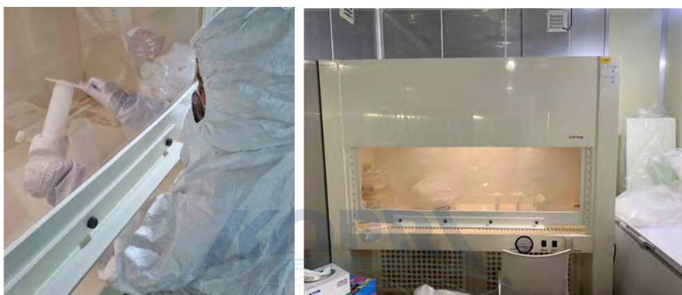
Fig 5.2. Chiselling procedure of the portions of Styx-M ice core for trace elements analysis and the class 100 clean bench in a cold room at KOPRI.
