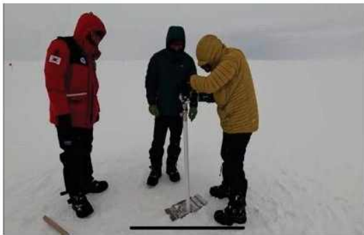
Figure 13. Hand Auger drilling
