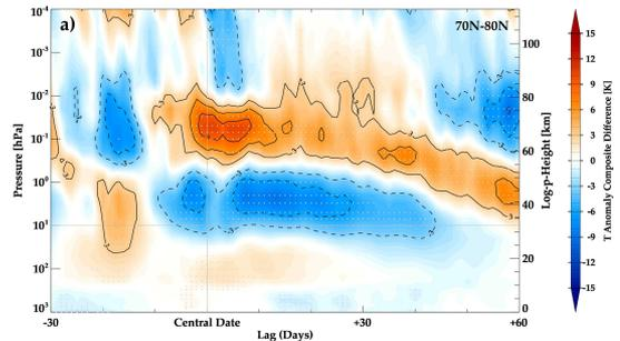
Figure 2. Composite differences between split type and displacement type of temperature anomaly averaged over  $70^{\circ}\text{N}-80^{\circ}\text{N}$  for WACCM. The light gray dots indicate 95% significant regions according to student's t-test.
