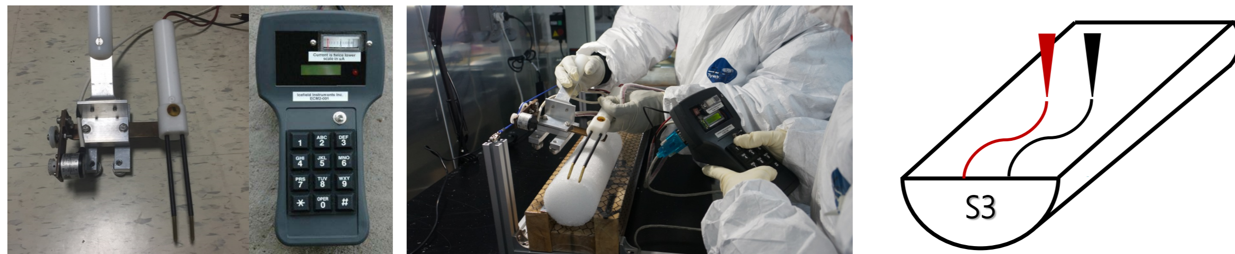
Fig. 3. The ECM instrument used (Portable ECM unit, Icefield Instruments Inc. Canada) consists of two electrodes with 20 mm spacing. Two electrodes are dragged in a zig-zag (to minimize the influence of air bubbles and other causes of poor contact) at voltage of 1000 VDC. A trimming blade used to prepare a fresh, flat surface along the length of the core (measured at -14 \text{ }^\circ\text{C} \pm 2 ). It was measured 3 times to calculate the representative values. The spatial resolution of the measurement is about 5 mm.
