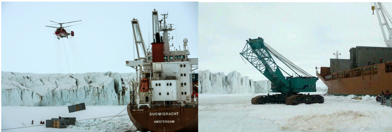
Figure 2: Unloading from the cargo ship, MV SUOMIGRACHT , using a heavy helicopter and unloading of the heaviest cargo, a 100 ton crawler crane.
