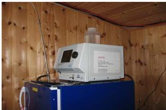
Figure 3. Aerosol Particle Counters (CPC) with different cutoff diameters installed at the Corbel station
