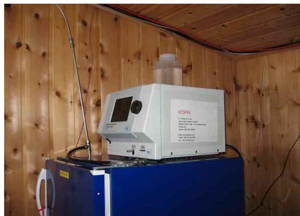
Figure 3. Aerosol Particle Counters (CPC) with different cutoff diameters installed at the Corbel station
