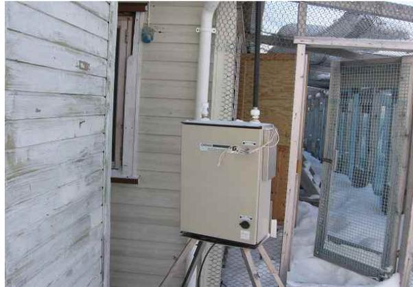
Figure 4. An Optical Particle Counter (OPC) installed at the Grubadet station.
