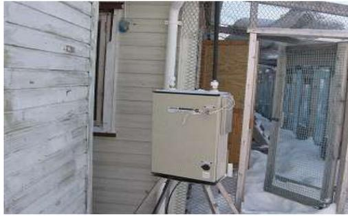
Figure 4. An Optical Particle Counter (OPC) installed at the Grubadet station.
