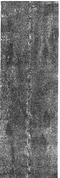
Fig. 9 A side-scan sonar sonogram showing pockmarks (black) probably formed by fluid and/or gas discharge.
