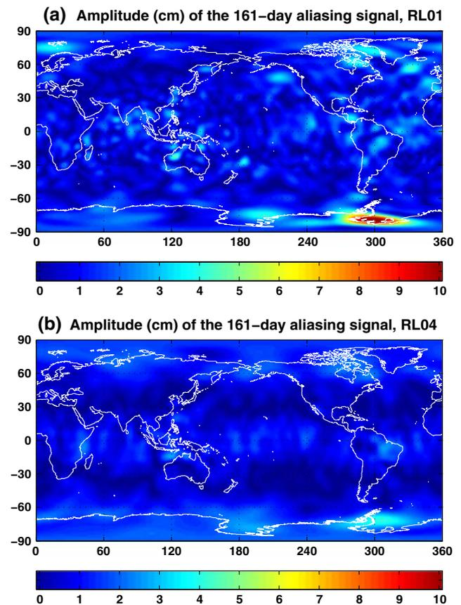
**Fig. 1** **a** Least square fit amplitude (cm of equivalent water height) of the 161-day S<sub>2</sub> alias from the 53 monthly GRACE solutions in RL01. **b** As in **a** but for RL04
