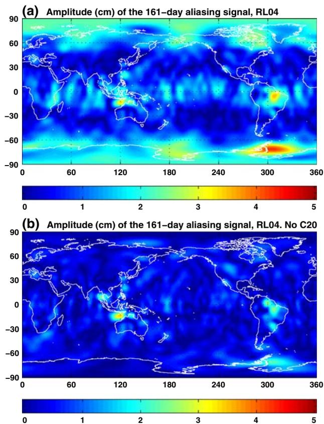
**Fig. 6** **a** Amplitudes (cm of equivalent water height) of the 161-day alias signal from 53 CSR RL04 monthly solutions with  $C_{20}$  included (same as Fig. 1b, but different color scale). **b** As in **a**, but with  $C_{20}$  excluded
