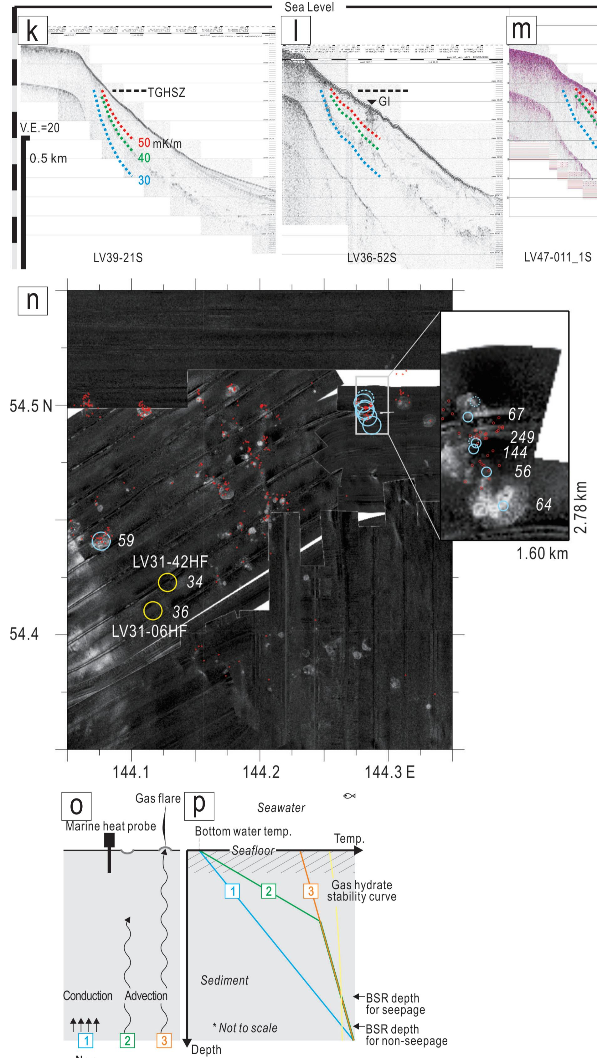
[k], [l], [m] Seismic profiles showing the bottom-simulating reflectors (BSRs). The Dotted curves represent estimated BSRs based on geothermal gradients of 30 (blue), 40 (green) and 50 (red) mK/m using the stability curve by Tishchenko et al. (2005). The horizontal lines indicate the top of gas hydrate stability zone (TGHSZ). Gas hydrate sample was taken at Gisella seepage structure (GI, reverse triangle), which is shown in [c]. See [c] for the location of the echosounder profiles.
