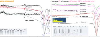
Representative ATR spectra of and elemental concentrations of 5 individual particles of sample those show the coexistence of feldspars ((Na,K,Ca)AlSi<sub>3</sub>O<sub>8</sub>) and SiO<sub>2</sub> (felsic materials) where silica content is less than 20% indicating presence of volcanic basalt.
