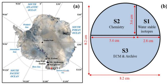
**Fig. 1.** (a) The GV7 drilling site (70°41'S, 158°52'E; elevation 1950m) (b) Ice core sectioning strategy as defined by the GV7 Ice core (Depth: 78 m).
