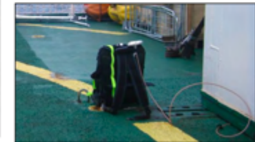
GPS antenna for the GT-1A while the AS350 was hangered. The rigid framed backpack strapped to the helo deck proved to be adequate as an antenna
