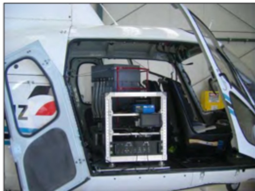
GT1a Power electronics and GPS receiver
