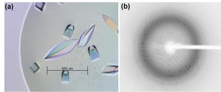
Figure 3. Crystal morphology and diffraction pattern of recombinant FfIBP. (A) FfIBP crystals grown with 0.1M sodium acetate pH4.4 and 3M sodium chloride. (B) X-ray diffracted image (2.9 Å resolution) obtained during data collection from the FfIBP crystal.
