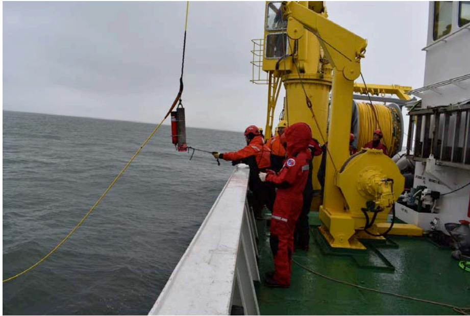
Figure 6.5 Photograph showing the clump weight being attached to the ROV tether. The clump weight also has a USBL beacon attached to it.
