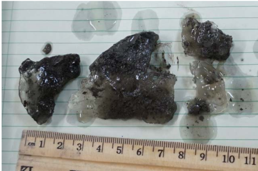
Figure 8.3: Ice fragments from the bottom of core ARA08C-06-GC01 collected from the top of a shelf edge pingo west of the Mackenzie Trough.
