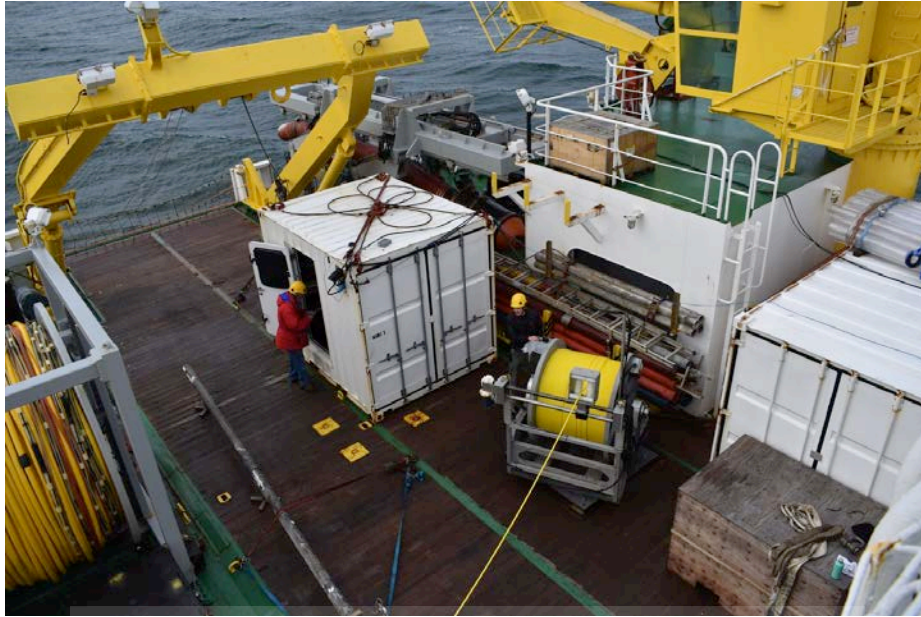
Figure 6.1 Location of ROV control room and winch on the aft deck of the Araon.
