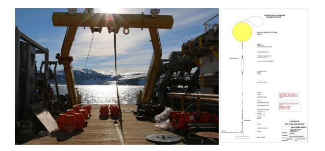
Figure 2: Left, floats and mooring line splayed out on fantail of R/V Araon. Right, detailed diagram of moorings deployed near Drygalski ice shelf.
