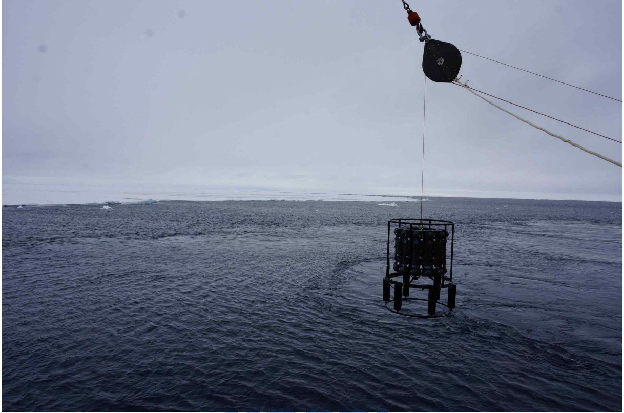
Fig. 3.3.3. A picture showing the sampling of metal free seawater using Go-FLO rosette system for iron assimilation experiment.
