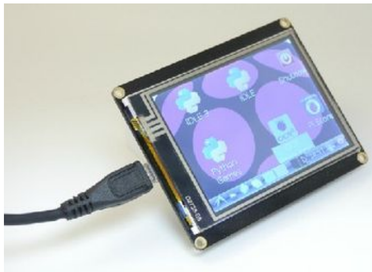
Fig 5. Touch screen for Raspberry PI 2
