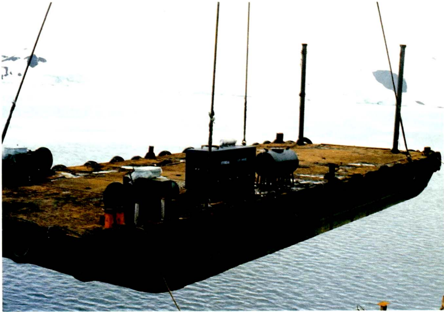
Fig. 4. Flat for temporary wharf.
