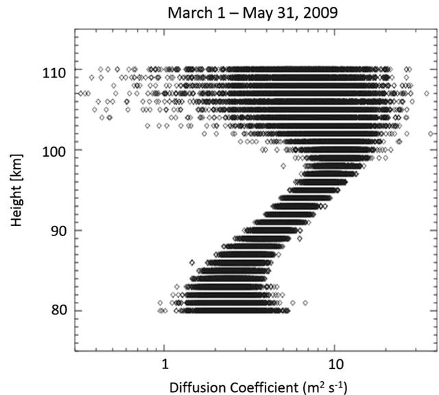
**Fig. 4** Height profiles of the observed meteor diffusion coefficient from March to May, 2009 at King Sejong Station in Antarctic. Each point represents a 30-min average of the observed values
