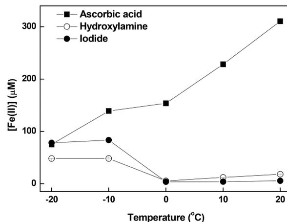
**Figure 6.** Temperature effect on the production of Fe(II) dissolved from goethite in the presence of ascorbic acid, iodide, and hydroxylamine. Experimental conditions: [goethite], 0.2 g/L; [ligand], 1 mM; reaction time, 24 h; and pH, 3 (the error bars are smaller than the symbol size).
