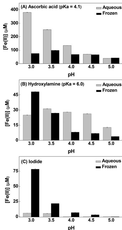
**Figure 3.** pH-dependent dissolution of ferrous iron from goethite in aqueous (gray) and frozen (black) solutions in the presence of (A) ascorbic acid, (B) hydroxylamine, and (C) iodide. The pH values indicate the pH of the aqueous solution before freezing. Experimental conditions: [goethite], 0.2 g/L; [ligand], 1 mM; and reaction time, 24 h.
