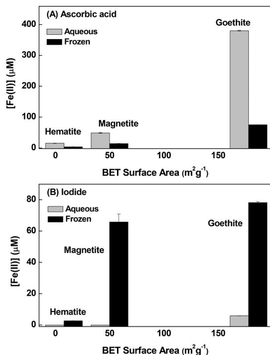
**Figure 2.** Dissolution of ferrous ions from three kinds of iron oxides having different surface areas in aqueous (gray) and frozen (black) solutions at pH 3 in the presence of (A) ascorbic acid and (B) iodide. Experimental conditions: [iron oxide], 0.2 g/L; [ligand], 1 mM; and reaction time, 24 h.
