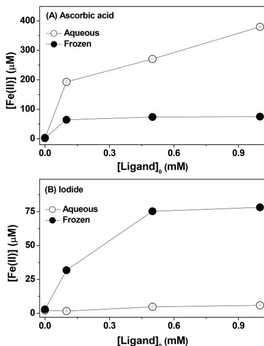
**Figure 7.** Dissolution of Fe(II) from goethite in aqueous and frozen solutions as a function of the ligand concentration: (A) ascorbic acid and (B) iodide. The ligand concentration indicates the aqueous concentration before freezing. Experimental conditions: [goethite], 0.2 g/L; reaction time, 24 h; and pH, 3 (the error bars are smaller than the symbol size).
