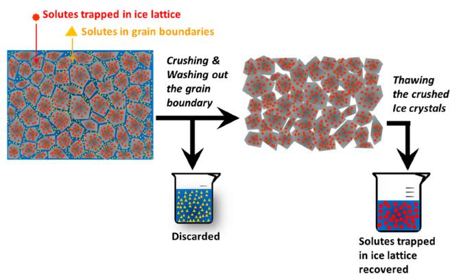
**Figure 4.** Illustration of the experimental procedure for estimating the concentrations of solutes (ligands) trapped in ice lattice.
